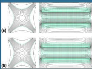
Figure 5: Equipotential contours in  $xy$  plane (left) and  $zy$  plane (right) for (a) DLP LIT with  $r_{ox} = r_{oy} = 2.526$  mm and (b) DLP LIT with  $r_{ox} = 3$  mm and  $r_{oy} = 2.526$  mm.
