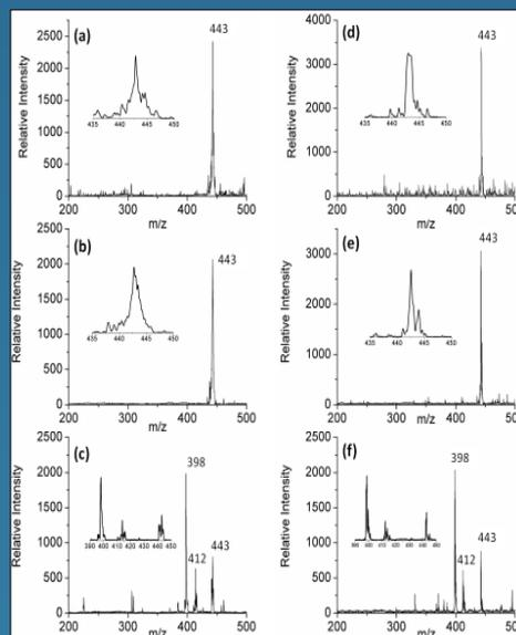
Figure 7: Mass spectra of rhodamine B collected using the DLP LIT (a,b,c) and spectra obtained using a conventional RIT built by Purdue University operating under identical conditions (d,e,f). The rf voltage corresponding to  $m/z 443$  was  $717 V_{pp}$  for DLP LIT and  $2280 V_{pp}$  for RIT.
