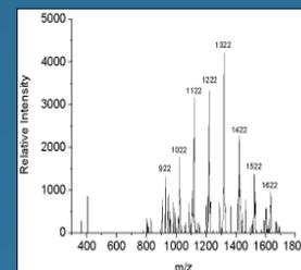
Figure 9: Mass spectrum of Ultramark obtained from Mini 10 and the DLP LIT. The drive parameters include rf amplitude of approximately  $2670 V_{pp}$  and rf frequency of  $990$  KHz.
