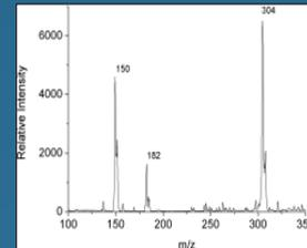
Figure 8: Mass spectrum for 5 ppm mixture of cocaine and methamphetamine. Protonated methamphetamine and cocaine are observed at  $m/z 150$  and  $304$ . The peak at  $m/z 182$  corresponds to a fragment of cocaine.
