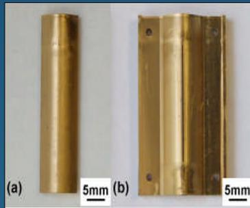
Figure 3: Photographs of the DLP LIT components showing gold coated individual electrodes (a) y electrode, (b) x electrode.
