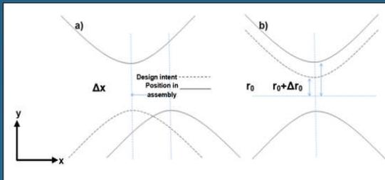
Figure 4: Design drawing for DLP LIT electrode positioning in assembly.
