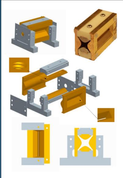
Figure 2: DLP LIT prototype with CAD model and exploded assembly.
