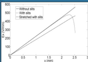
Figure 6: Electric field variations in  $x$  direction from the center of the DLP LIT to the electrode edge with  $716 V_{pp}$  rf amplitude. Variations were done with original  $r_{ox} = 2.526$  mm.
